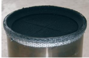
The same DPF, after hours of stop-&-go driving and idling - Massive amount of unburned collected soot.
