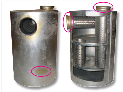
Turkish competitor: The thin materials show beginning of a tearing process after only 30 minutes testing.
