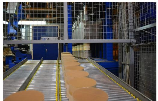
*Robotized wash coating for high volume production*
