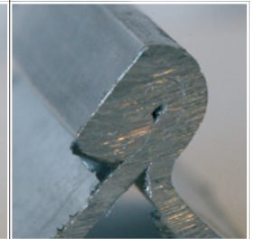
Dinex: Stronger closing of the lockseam
